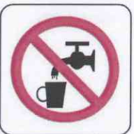
SP-010 AGUA NO POTABLE
